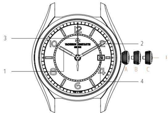
I. I Winding, time-setting and correction crown
